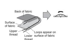
**Solution:** Reduce the tension by turning the upper
