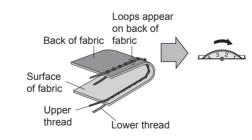
**Solution:** Increase the tension by turning the upper tension control dial to a higher number.
