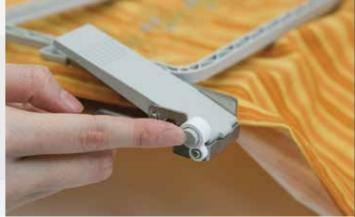
Re-hoop your fabric without removing the frame. Just release the latches, slide the fabric to the next embroidery position, and relock.
